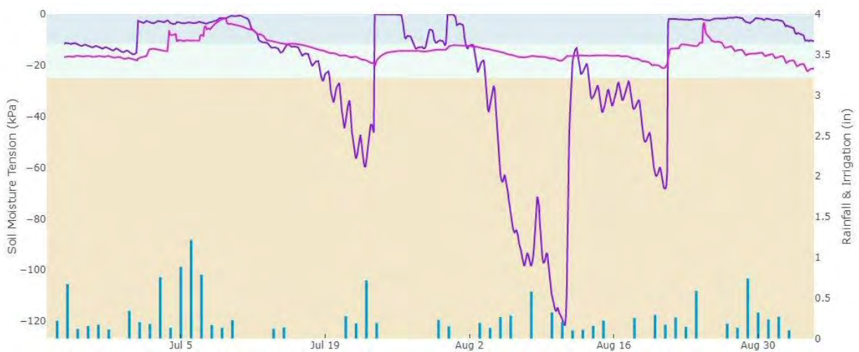
Graph of data from SMSS installed in Thomas County cotton field in 2020. Shallow sensor shown in dark blue, deep sensor shown in purple.
