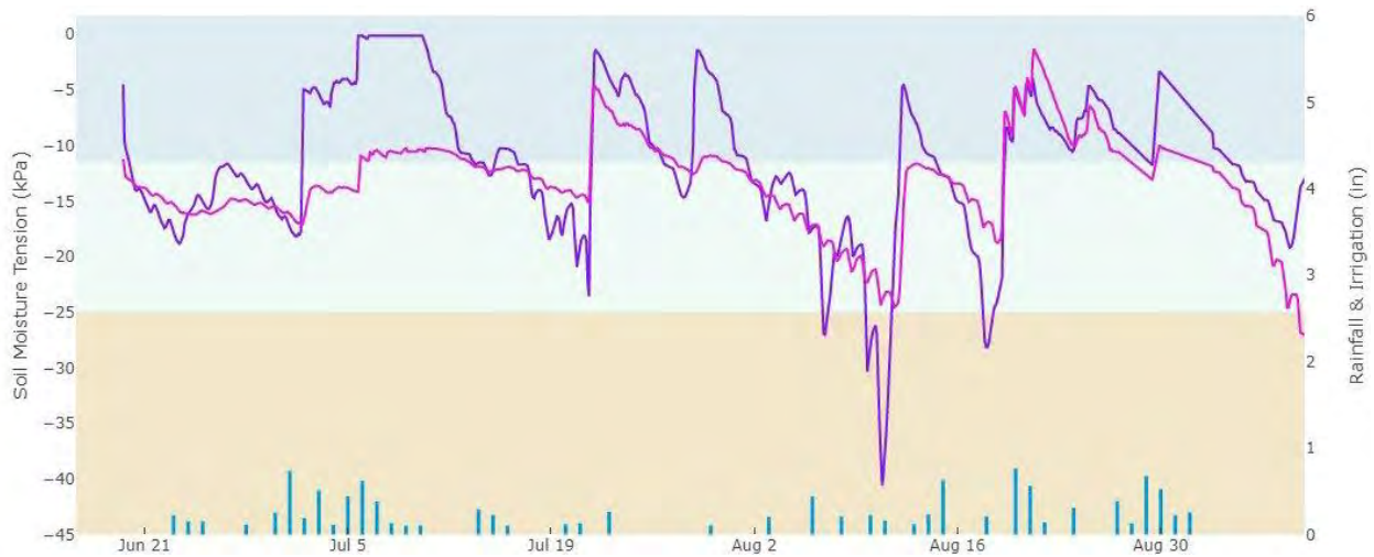
Graph of data from SMSS installed in Miller County cotton field in 2019. Shallow sensor shown in dark blue, deep sensor shown in purple.
