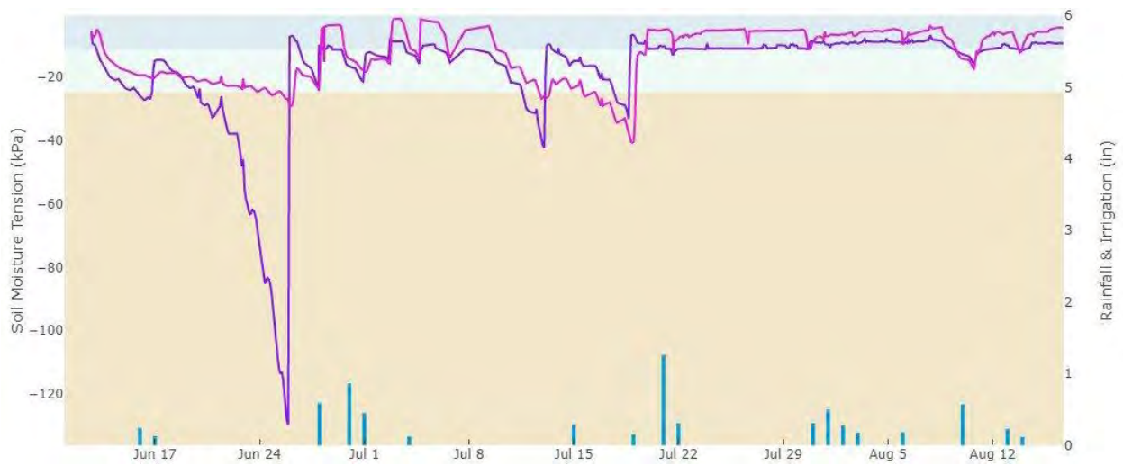
Graph of data from SMSS installed in Mitchell County cotton field in 2020. Shallow sensor shown in dark blue, deep sensor shown in purple.
