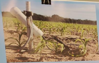
Figure 1: A UGA SSA soil moisture sensor node consists of a large antenna, a probe with three sensors, and a computer board. The probe collects moisture readings at three different depths, relays them to the computer which then uploads them to a cloud server.
