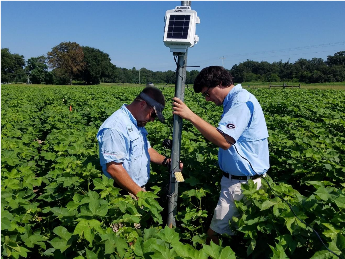
Above: B.J. & Cale installing Davis Instr. node in Dr. Kemerait's cotton study. Below: BJ installing Davis Instrument "repeater" node on top of roof.
