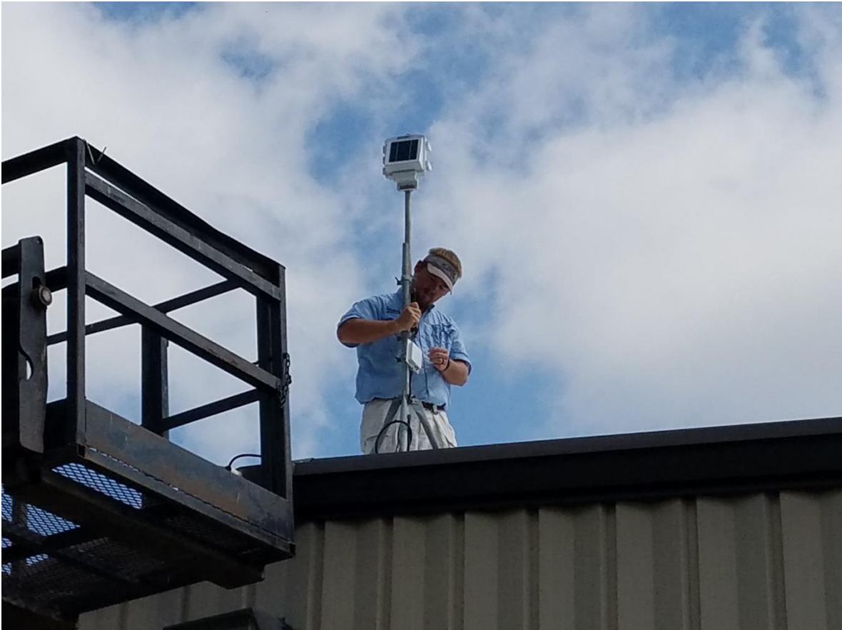
Above: B.J. & Cale installing Davis Instr. node in Dr. Kemerait's cotton study. Below: BJ installing Davis Instrument "repeater" node on top of roof.
