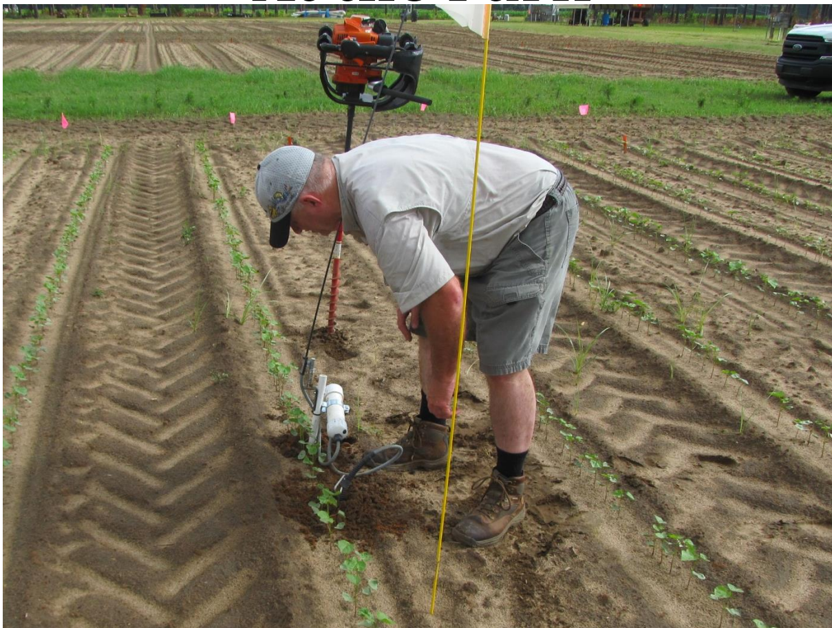
Above: Mike Tucker installing soil moisture sensors in field. Below: Dr. Vellidis' crew setting up Smartfield camera.
