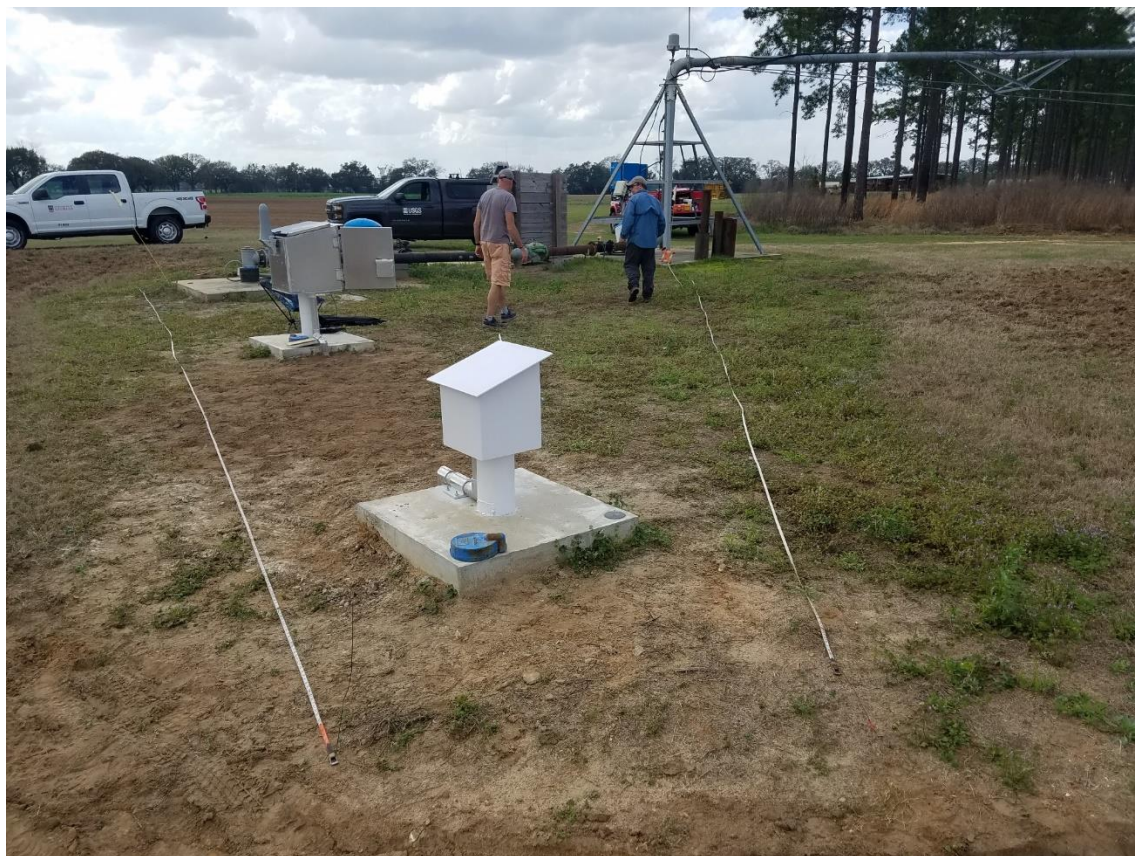
Above: Processing Dr. Vellidis' core samples from Newton lateral corn plots. Below: USGS installed sensors and logger to monitor the Claiborne and Floridan wells.
