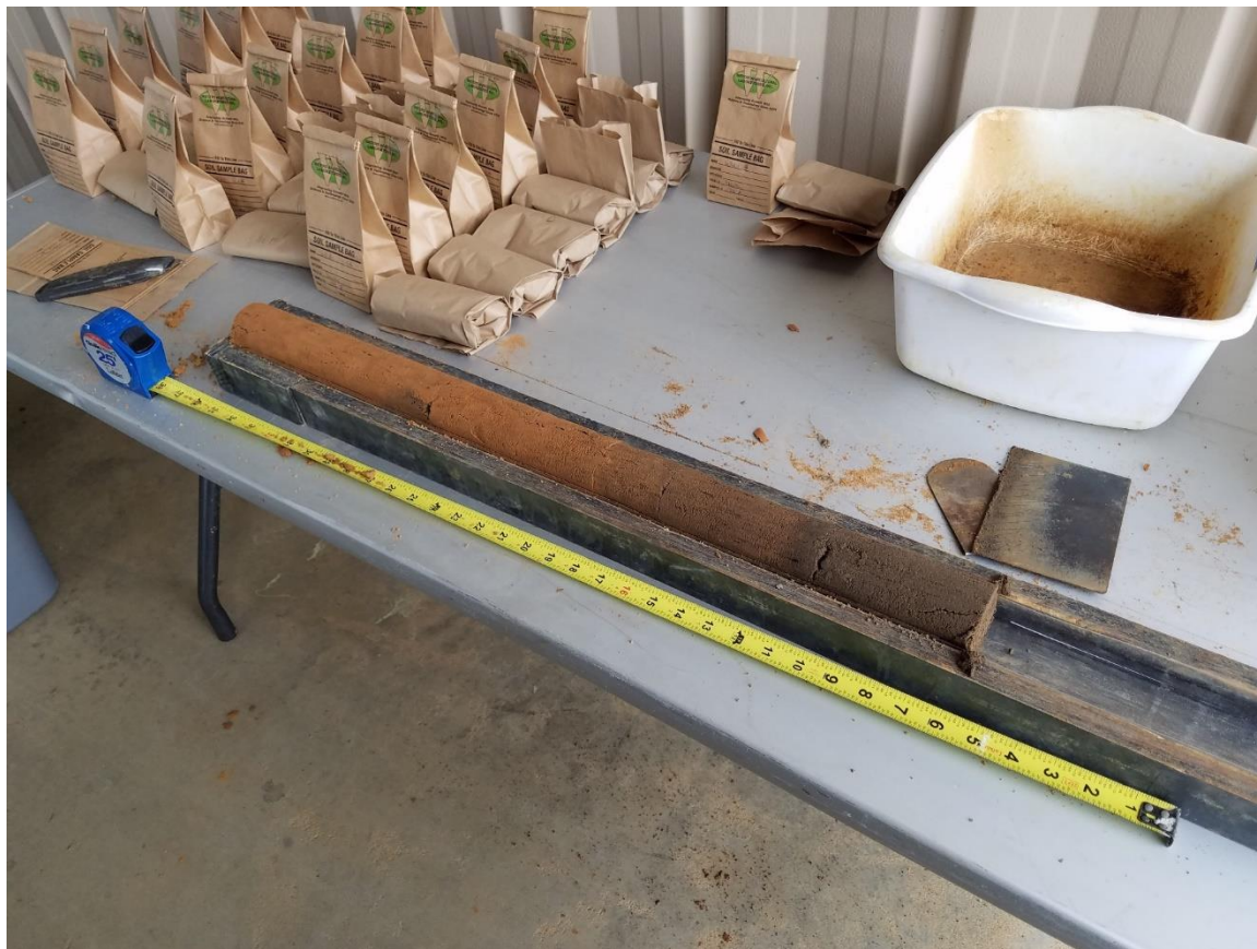
Above: Processing Dr. Vellidis' core samples from Newton lateral corn plots. Below: USGS installed sensors and logger to monitor the Claiborne and Floridan wells.
